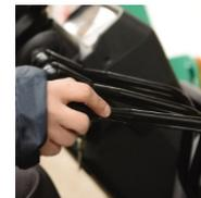
**Cowl-mounted hydraulic levers** provide easy-to reach easy-to-use control of mast operations.
