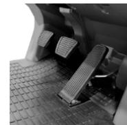
**Automotive-style pedals** with optimum pedal angle are easy to use and give good control without leg strain.
