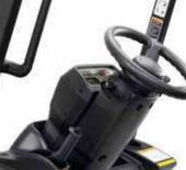
Adjustable Steering: The forklift's steering column is equipped with standard memory tilt steering. Allowing for infinite adjustment in a 12 degree range, the steering column's "memory" feature retains the operator's preferred settings for added convenience and comfort during operation.
